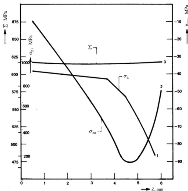
Figure 10. The change of characteristic stresses from central plane to surface.
