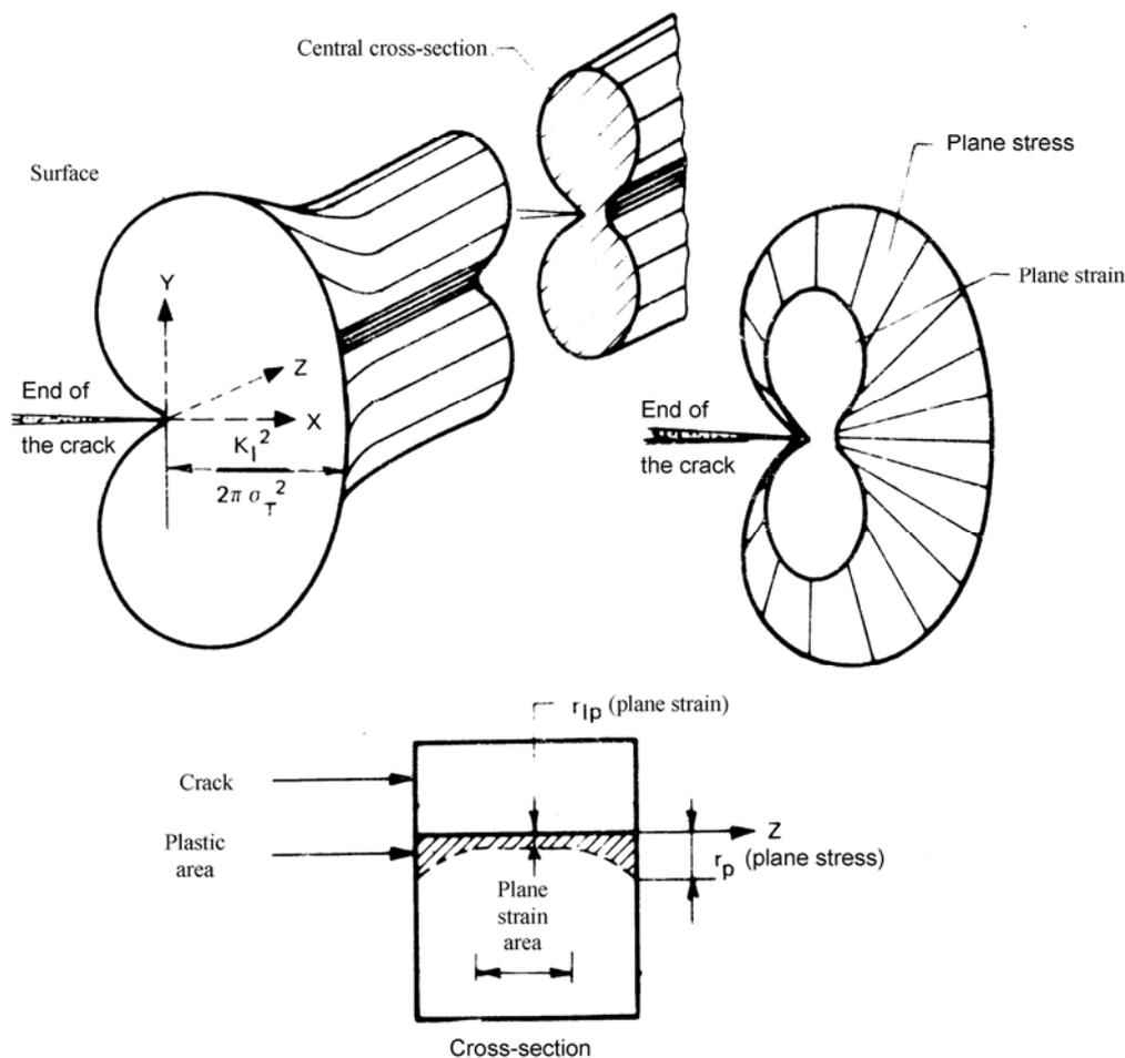
Figure 6. Plastic area around the crack tip.
