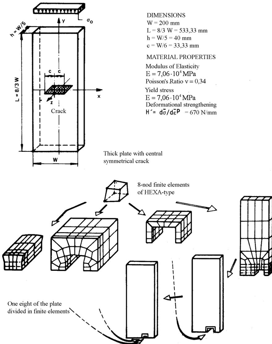
Figure 7. A plate with central crack, divided into finite elements.
