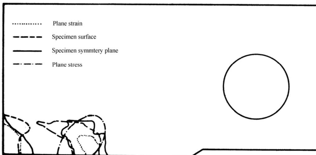
Figure 9. Comparison of plastic zones for plane strain and the centre of specimen, for plane stress and specimen surface.
