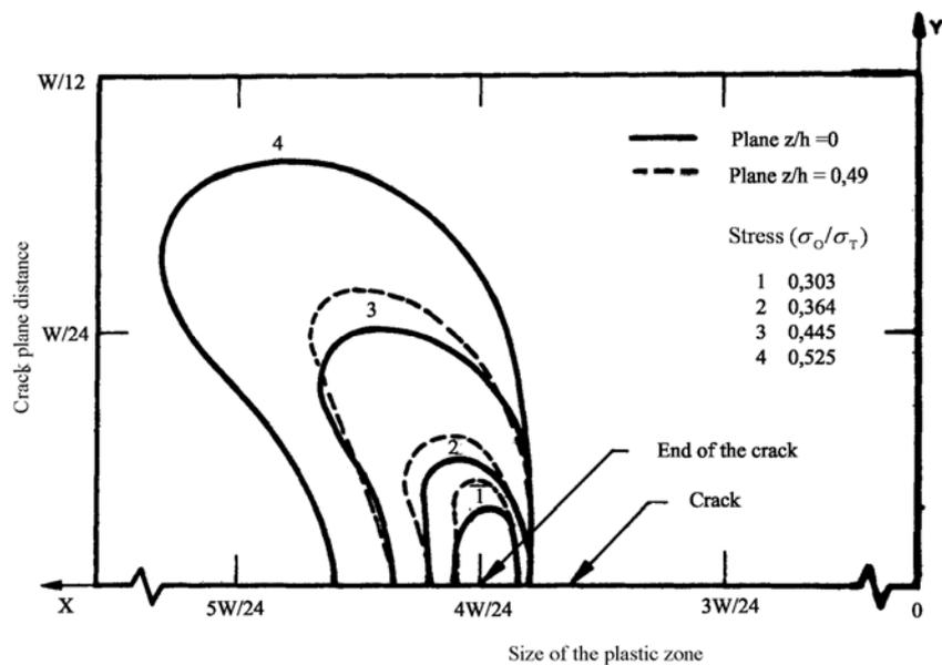
Figure 8. Size and shape of the plastic zone of the panel from Fig. 7.
