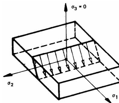
Figure 4. Maximum shear stress.
