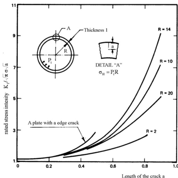
Figure 11. Change of stress intensity factors with crack entail and vessel radius.
