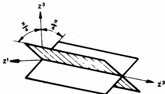
Figure 1. Planes of maximum shear stress.
