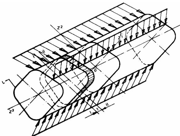
Figure 2. Plane strain state.
