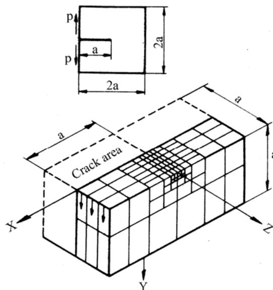
Figure 1. Compact specimen for tensile testing.
