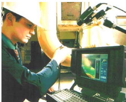
Slika 9. Ispitivanje kolena cevovoda pomoću \mu+ (video kamera) Figure 9. C-scan inspection of a pipe bend (video tracking).
