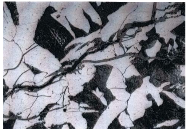
Slika 7. Mikrostruktura oko prsline (x 500) Figure 7 – Microstructure around the crack (x500)
