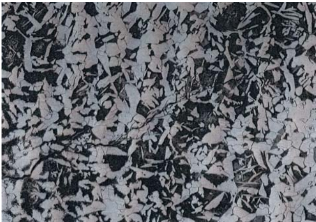
Slika 6. Mikrostruktura oko prsline (x 100) Figure 6 – Microstructure around the crack (x100)
