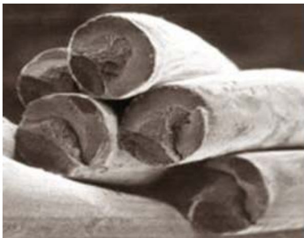
Slika 6. Zamorne prsline na mestu kontakta pojedinačnih žica. Inicirane prsline se vide nakon kidanja struka zatezanjem. Figure 6. Fatigue cracks at contact points of individual wires. Initiated cracks are visible after fracture of strand in tensile test.
