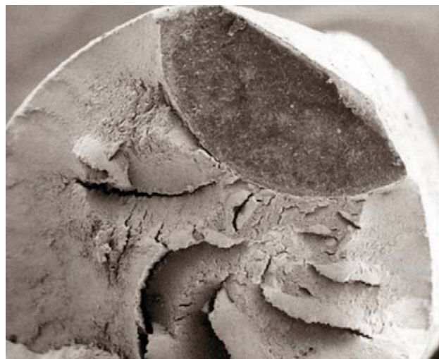
Slika 7. Zamorna prsline nastala na mestu dodira žice sa koturačom Figure 7. Fatigue crack initiated at the contact point with a sheave.
