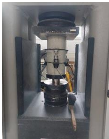
Figure 2. Measurement setup for determining the static modulus of elasticity using an extensometer.
