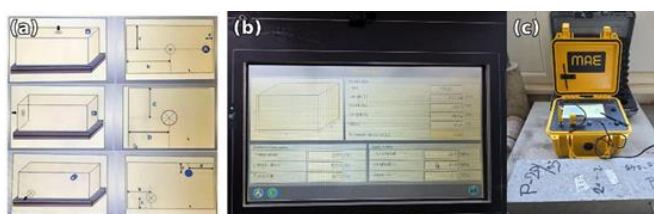
Figure 1. Resonance testing: a) measurement positions; b) measurement results and determination of dynamic elastic modulus; c) testing device (MAE C 311R system).
