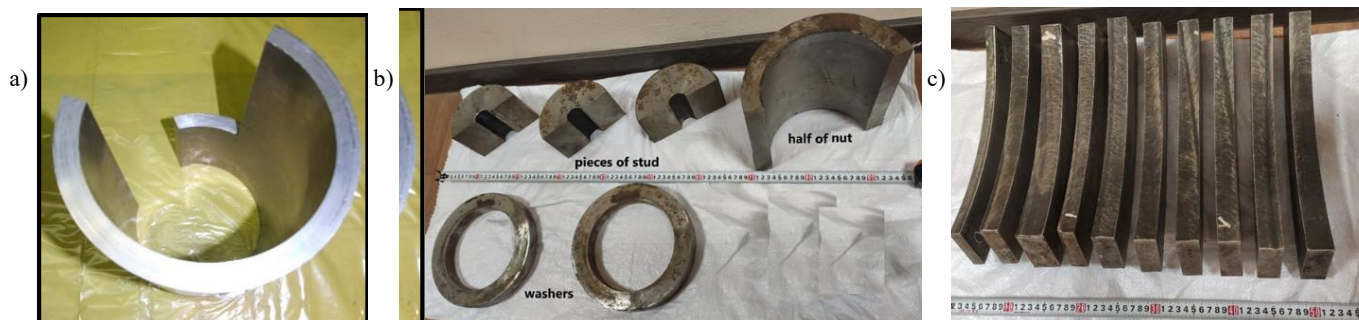
Figure 1. Materials selected for testing: a) pressuriser surge line 08Ch18N10T; b) WWER-1000 - reactor flange fastening parts 38KhN3MFA; c) WWER-1000 - main circulation piping 10GN2MFA.
