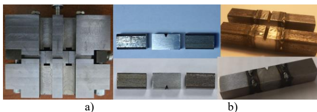
Figure 5. Charpy V-notch specimens: a) specialised alignment and welding jig; b) specimens reconstructed from broken halves.
