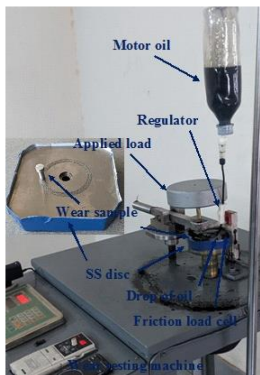
Figure 1. Photo of wear testing machine setup.
