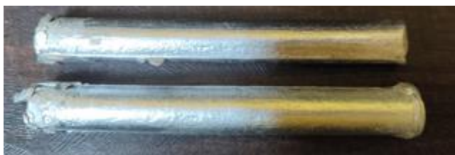
Figure 2. Al2005-B 4 C composites prepared.
