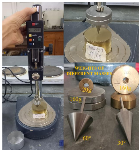
Figure 3. Fall cone test with weights of different masses and cones.
