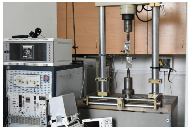
Figure 1. Experimental setup on the servo-hydraulic testing machine STM-100.
