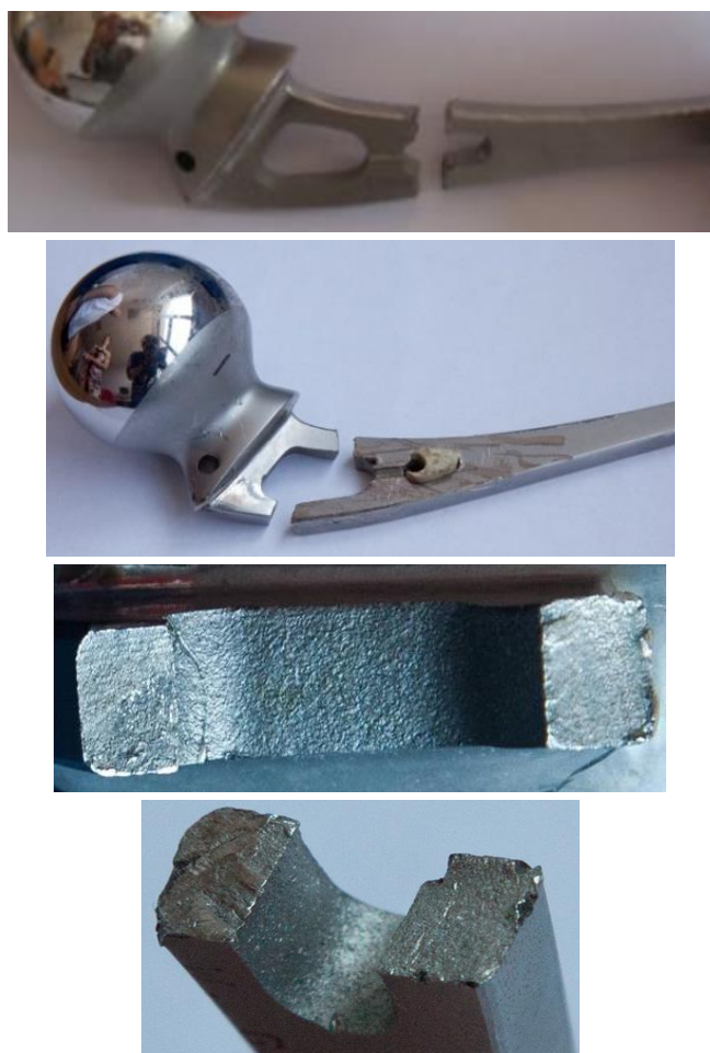
Figure 14. Examples of hip implant failure.
