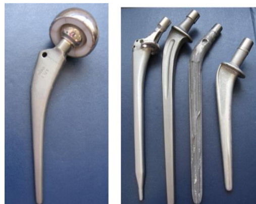
Figure 8. Geometry of real hip implant and different stem types
