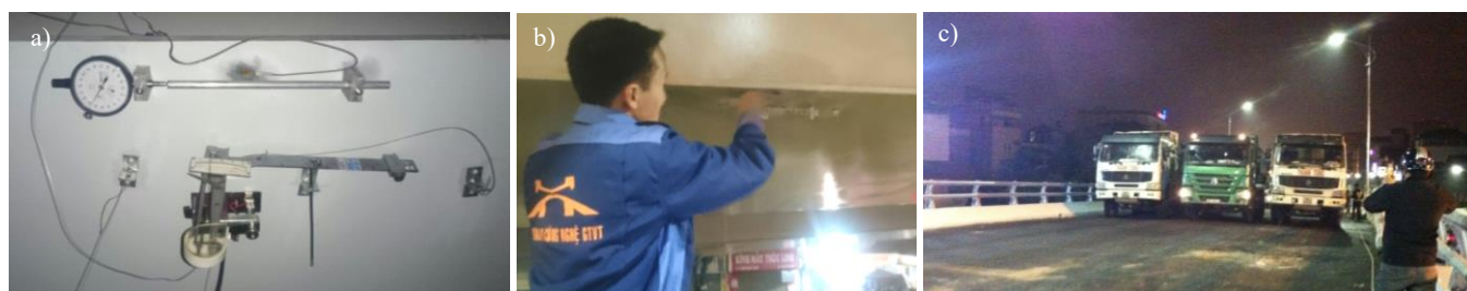
Figure 11. Loading the O Dong Mac bridge: a) b) installing steel box girder stress measuring device; c) arranging the load on the bridge.
