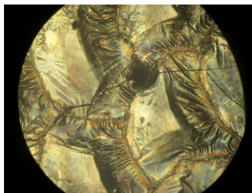
Figure 6. Surface of laser-treated sample with a crack after the first load cycles, \times 500 .
