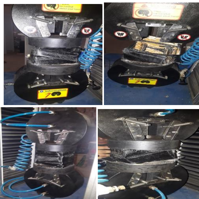
Figure 3. Delamination of crash box under a compressive test.
