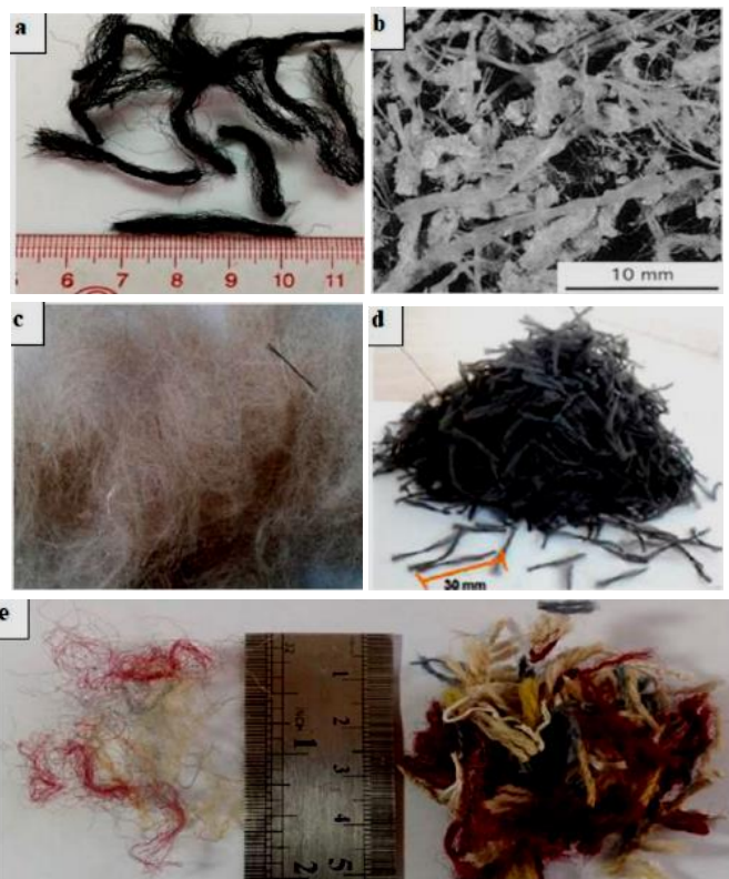
Figure 1. a) Chopped carpet fibres; b) carpet waste fibres under the microscope; c) carpet waste fibres; d) and e) size of used carpet waste fibres.
