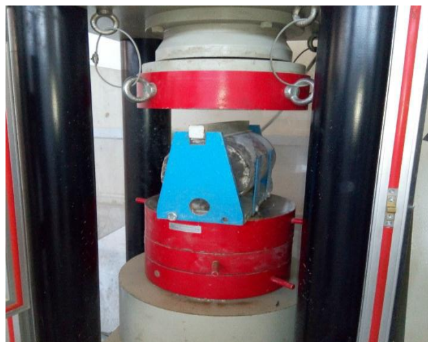
Figure 6. Tensile strength test device using the bisection method.
