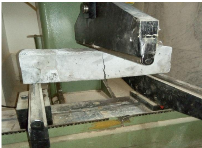
Figure 7. Flexural strength test with point loading in the centre.
