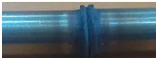
Figure 2. Profile of a friction weld joint.
