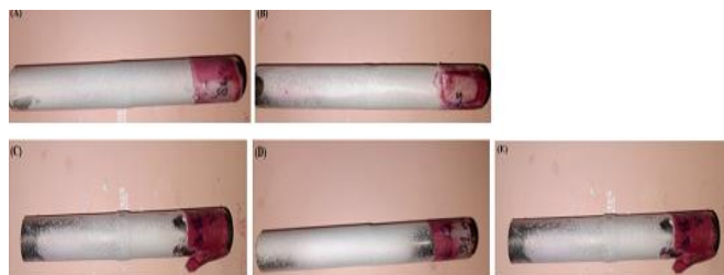
Figure 6. Penetrant joint inspection, conditions (A, B, C, D and E).
