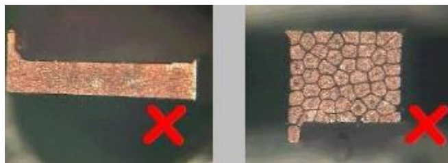
Figure 12. Microsection representation of welds with and without cutting edge.
