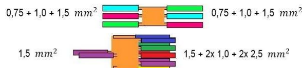
Figure 5. Symmetrical and asymmetrical connections for the inline splice.
