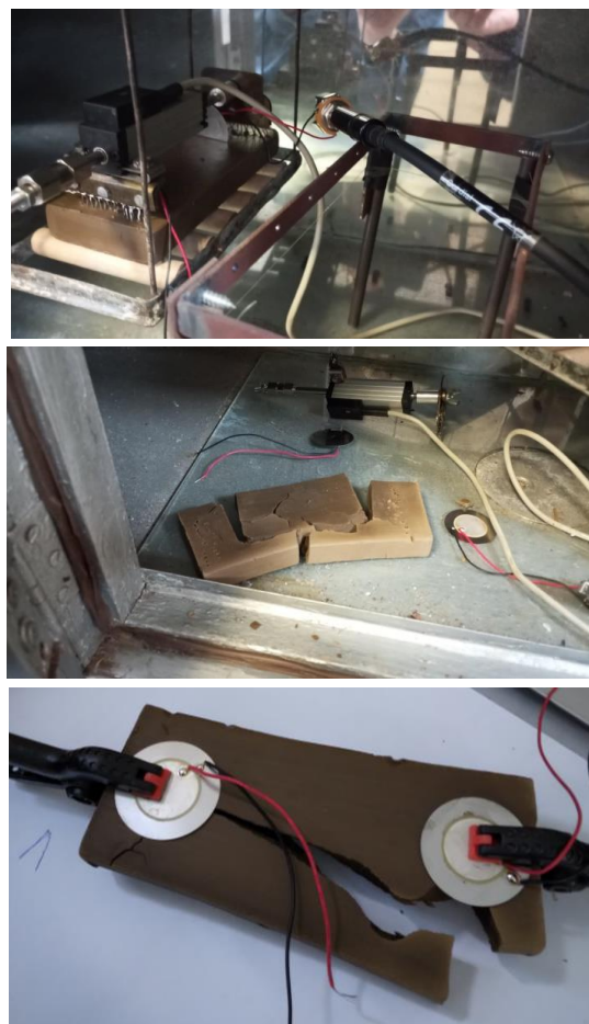
Figure 3. AE measurement setup - two sensors.
