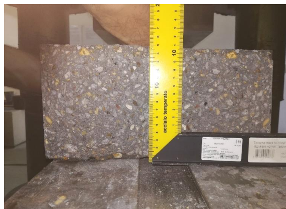
Figure 20. Depth of water penetration on experimental SCC sample.
