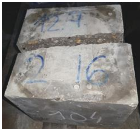
Figure 17. Crushed SCC sample after splitting tensile strength test.
