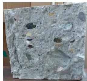
Figure 1. Laboratory concrete sample used in RCA production.
