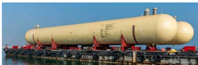
Figure 20. Bullet storage tanks, /20/.
