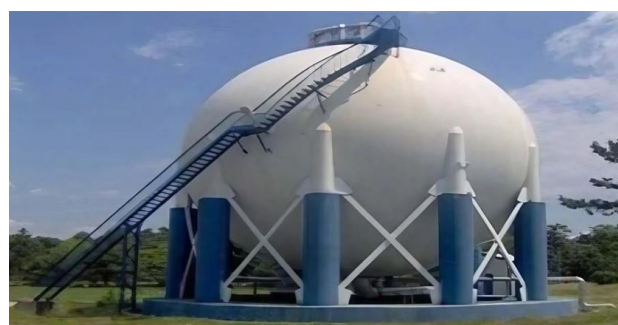
Figure 23. Elliptic tanks with a longer horizontal axis, /23/.
