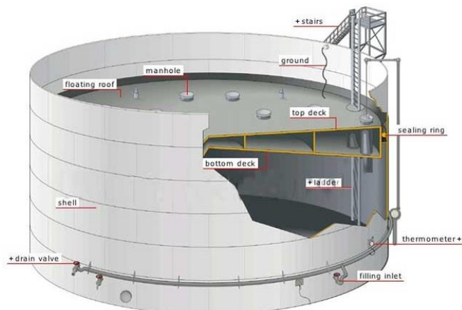
Figure 9. Double-deck floating-roof tank, /13/.
