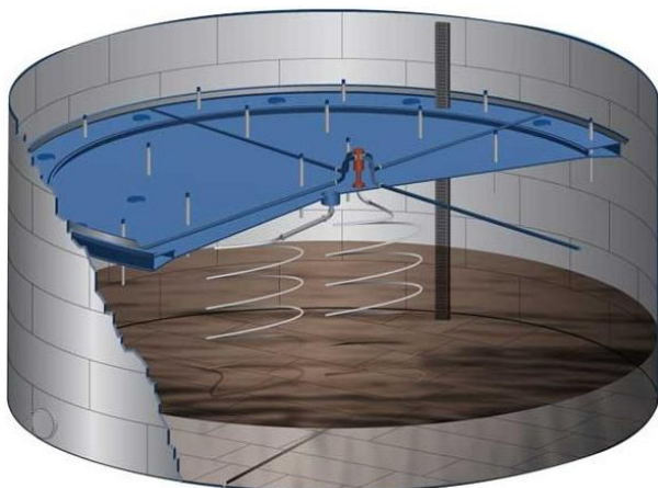
Figure 8. Annular-pontoon floating-roof tank, /13/.
