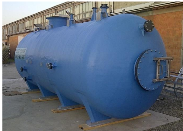
Figure 14. Storage tank supported on saddles, /15/.
