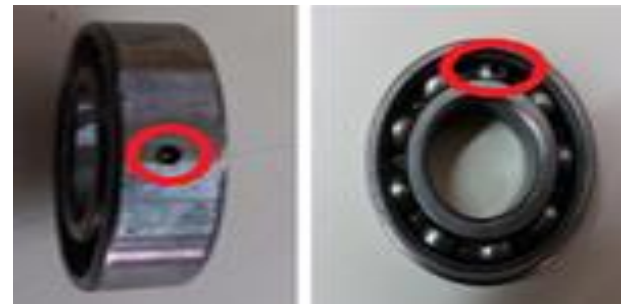
Figure 3. Bearing faults: outer race fault (left); cage fault (right).
