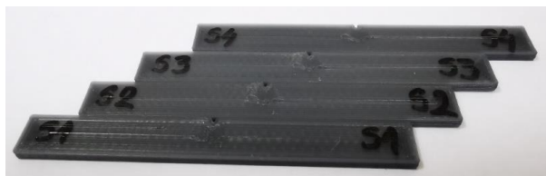
Figure 3. SENT specimens made by FDM technique from PLA material.
