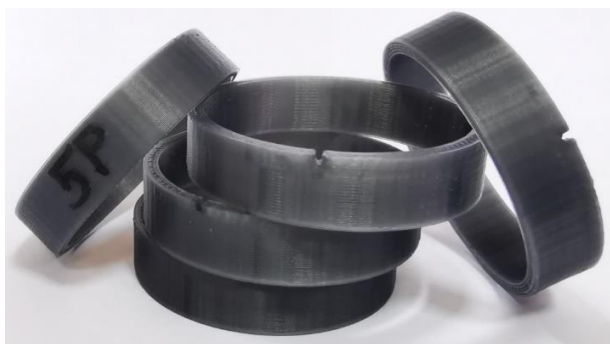
Figure 2. PRNT test specimens made by FDM technique from PLA material.
