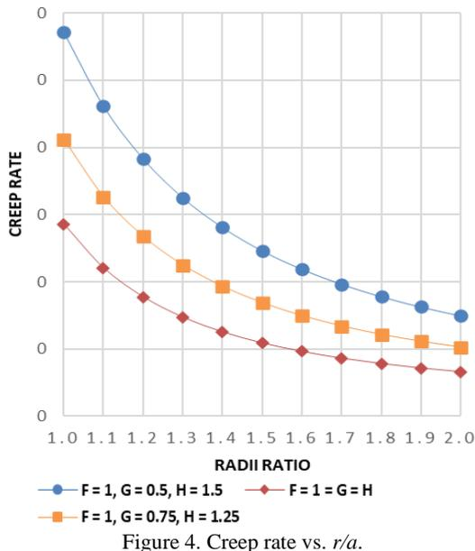
Figure 4 represents the creep rate decreases along the radius in plane stress condition, having only internal pressure. Here, also it may be seen that in plane stress conditions, creep rate is lower in isotropic cases as against the anisotropic cases. Which means that isotropic materials behave better than anisotropic materials in such plane stress conditions.
