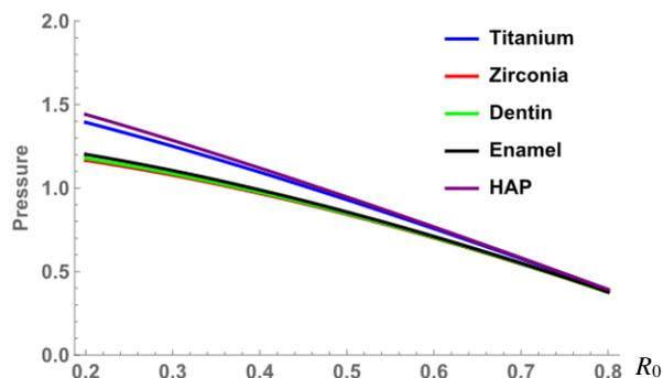
Figure 15. Initial pressure in the hemispherical crown for transversely isotropic materials.
