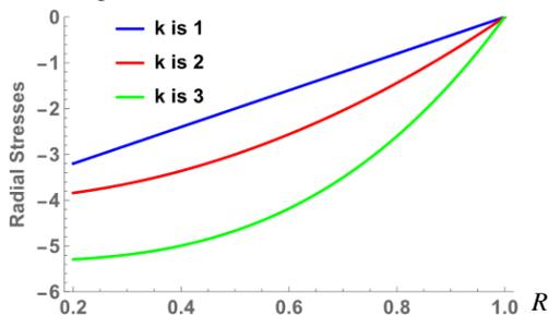
Figure 13. Radial stresses for fully plastic state in the hemispherical shell with different values of  $k$ .
