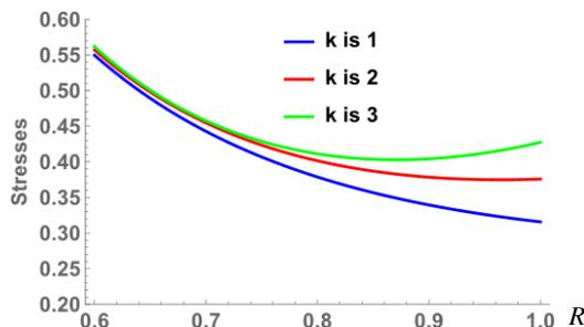
Figure 14. Circumferential stresses for fully plastic state in the hemispherical shell with different values of  $k$ .
