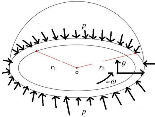
Figure 1. Geometry of hemispherical shell with external pressure.
