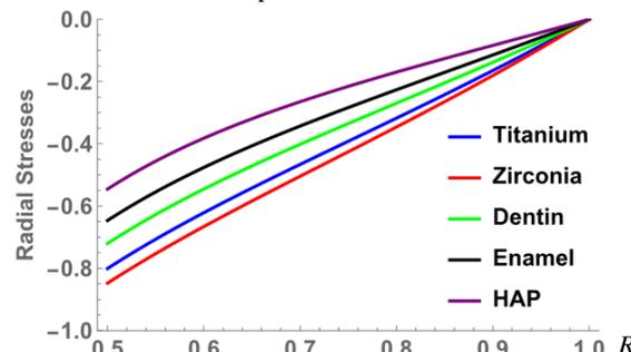
Figure 8. Radial stresses in the hemispherical crown for dental implant for  $k = 3$ .
