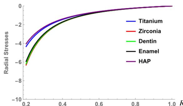
Figure 16. Radial stresses at initial yielding in the hemispherical crown for transversely isotropic materials.
