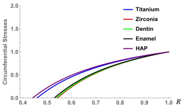
Figure 17. Circumferential stresses for initial yielding in the hemispherical crown for transversely isotropic materials.
