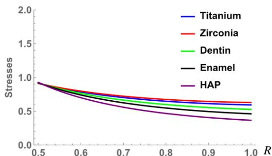
Figure 10. Circumferential stresses in the hemispherical crown for dental implant for  $k = 2$ .
