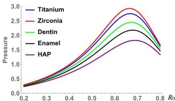
Figure 5. Initial pressure in the hemispherical crown for dental implant for  $k = 3$ .
