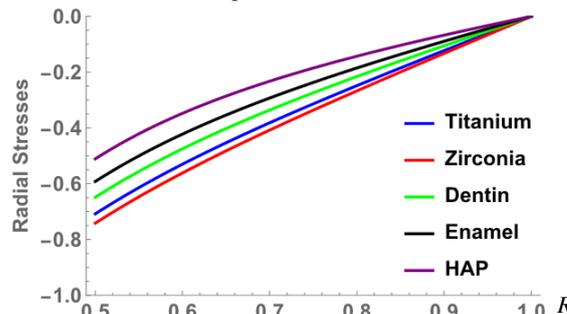
Figure 7. Radial stresses in the hemispherical crown for dental implant for  $k = 2$ .
