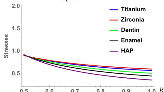
Figure 9. Circumferential stresses in the hemispherical crown for dental implant for  $k = 1$ .
