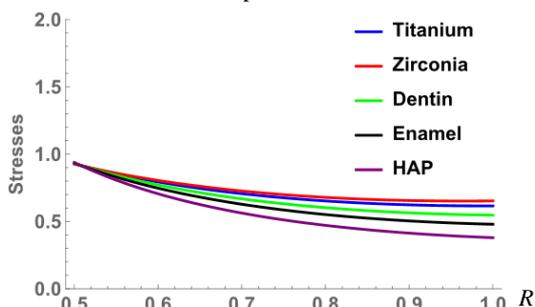
Figure 11. Circumferential stresses in the hemispherical crown for dental implant for  $k = 3$ .
