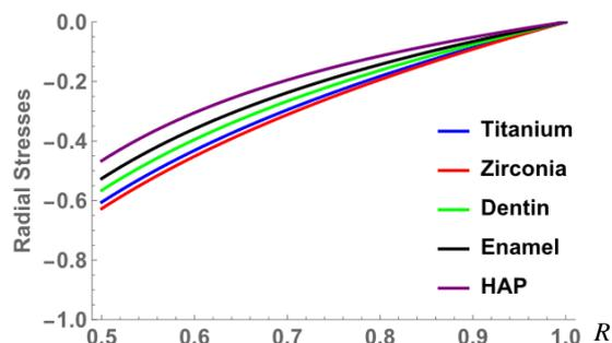
Figure 6. Radial stresses in the hemispherical crown for dental implant for  $k = 1$ .
