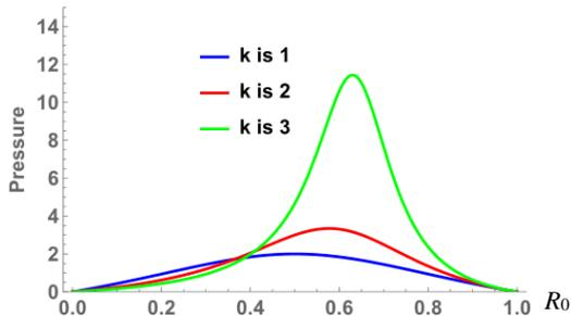
Figure 12. Pressure required at fully plastic state in the hemispherical shell with different values of  $k$ .
