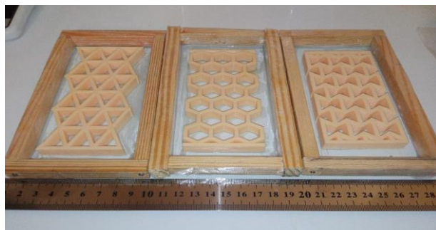
Figure 3. Positioned printed samples securely within a wooden mould.
