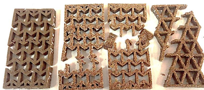
Figure 9. Samples of honeycomb after compression test.
