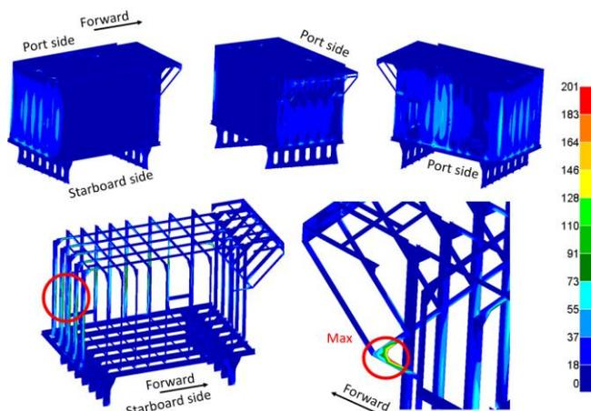
Figure 6. PS deckhouse Von Mises stress results for loading case 1 and scantling case 3.
