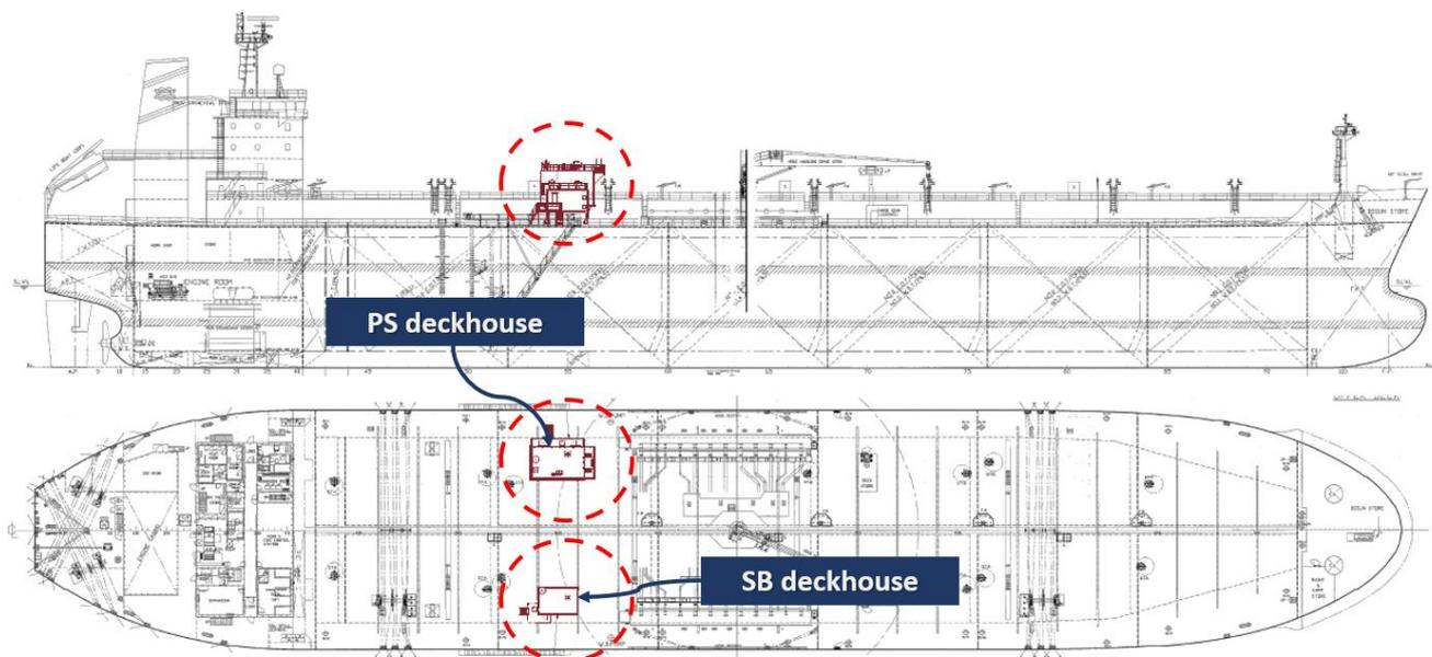
Figure 1. The extract from the general arrangement plan of one of the ships with marked locations for the deckhouses.
