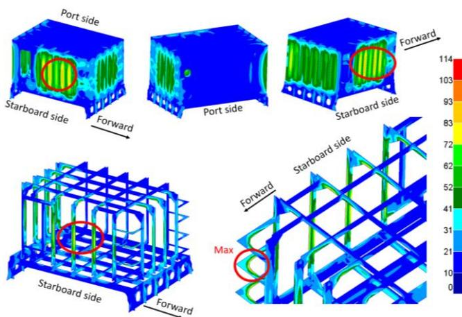
Figure 7. SB deckhouse Von Mises stress results for loading case 1 and scantling case 3.
