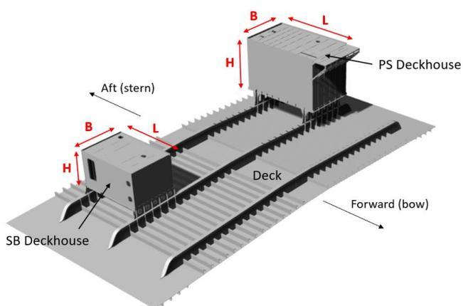
Figure 2. 3D model of deckhouses and part of the deck.
