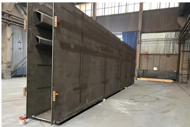
Figure 4. Large beam straightened.
