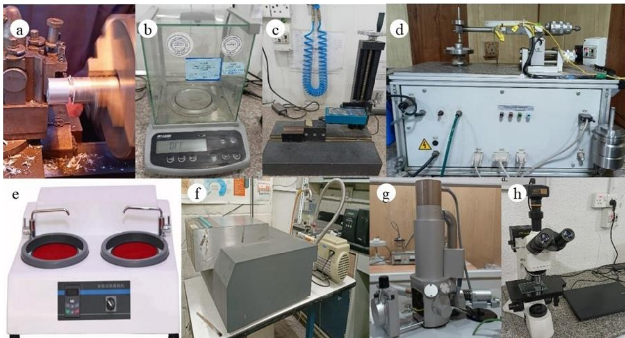
Figure 1. (a) Turing machine section to prepare specimen; (b) microbalance 120 gr. d = 0.1 mg capacity; (c) surface roughness tester; (d) micro test machine; (e) grinder polisher; (f) wavelength dispersive XRF spectrometer; (g) scanning electron microscope (SEM); (h) optical micrograph.
