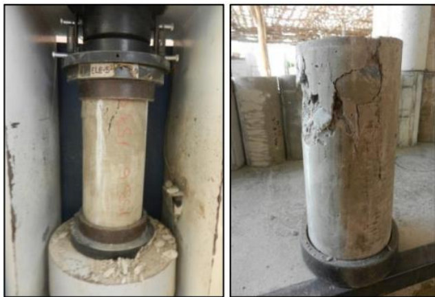
Figure 6. Specimen tested in axial compression.
