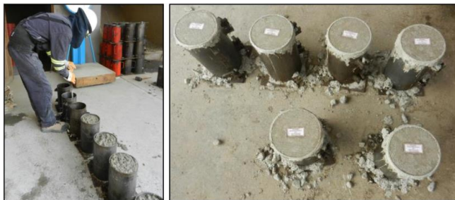
Figure 5. Production of concrete specimens.
