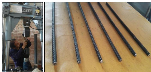
Figure 2. Placement of specimen in the jaws of universal machine. Tested specimens of 3/8" samples.
