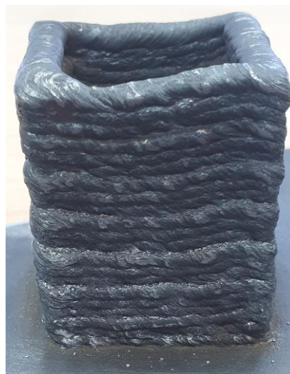
Figure 9. Metal structure in the form of a parallelepiped with wall thickness of 4 mm and height of 40 mm.
