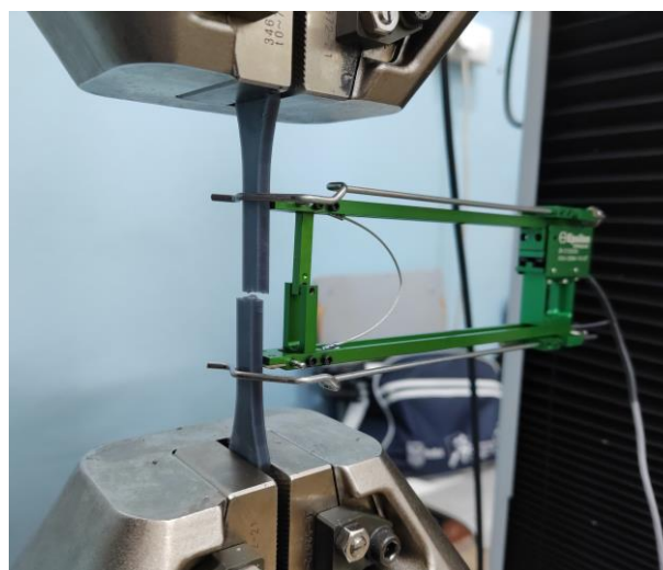
Figure 3. Tensile specimen after the test.
