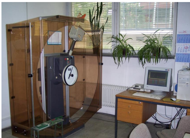
Figure 10. Instrumented Charpy pendulum WOLPERT 150/300J
