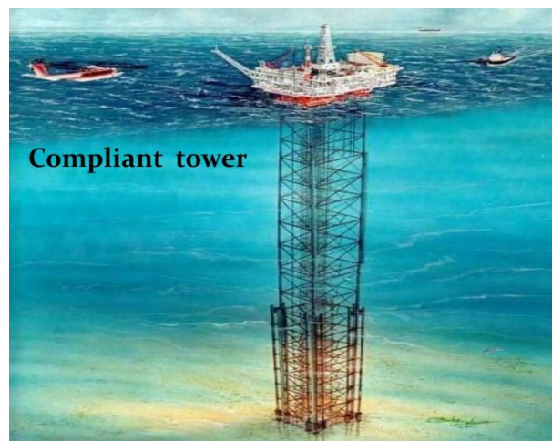
Figure 3 Platform for oil and gas type-Anchored tower /6/
