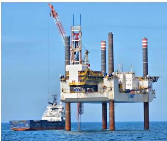
Figure 15 Height-adjustable oil rig with four column legs /27/.
