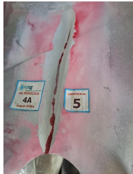
Figure 4. Groove on the Pelton runner's blade, made on the back side
