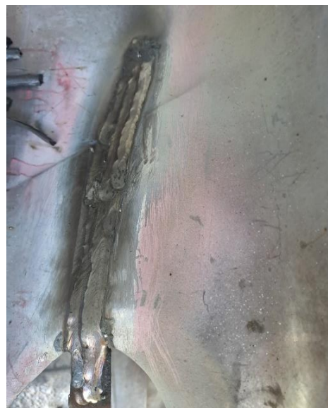
Figure 6. Blade groove after filling on the back side
