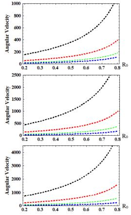
Figure 7. Angular velocity in initial yielding and fully plastic state with pressure 20 and temperature 0.1, 0.3, and 0.5, respectively.
