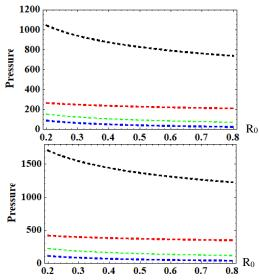
Figure 2. Pressure for initial yielding and fully-plastic state of transversely isotropic piezoelectric material and transversely isotropic material with angular velocity 20 and temperature 0.1, 0.3, and 0.5, respectively.
