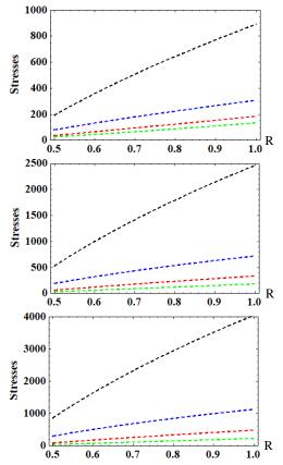
Figure 4. Circumferential stresses for piezoelectric and isotropic material steel with angular velocity 20 and temp. 0.1, 0.3, and 0.5, in respect.
