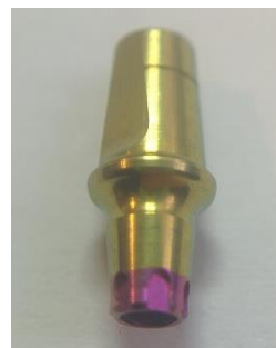
Figure 4. A standard transgingival abutment has a conical interface with an antirotational part (highlighted in purple).
