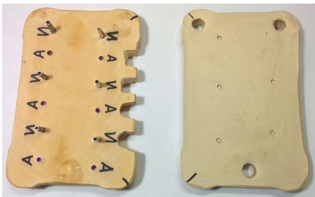
Figure 11. A plaster block made of class 4 gypsum with implants at right angles to the surface (a), and a mate (b).
