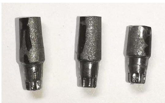
Figure 9. A group of abutments obtained by casting.
