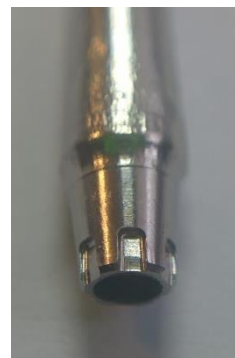
Figure 6. Surface of the conical interface of a milled abutment.
