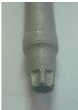
Figure 8. Surface of the conical interface of the SLS abutment.
