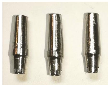
Figure 5. Individually made abutments by milling.
