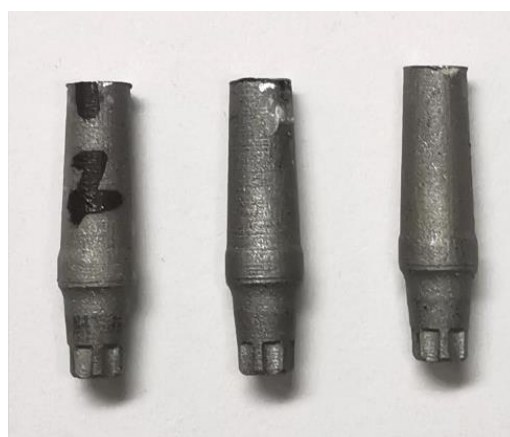
Figure 7. A group of abutments obtained by selective laser sintering (SLS).
