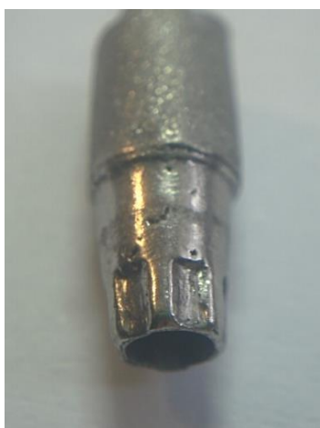
Figure 10. Surface of the conical interface of the cast abutment.
