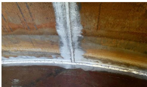
Figure 9. T-welded joint after cleaning and preparation for PT.
