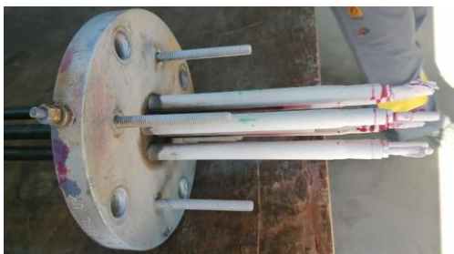
Figure 15. Penetrant test of electric heater.
