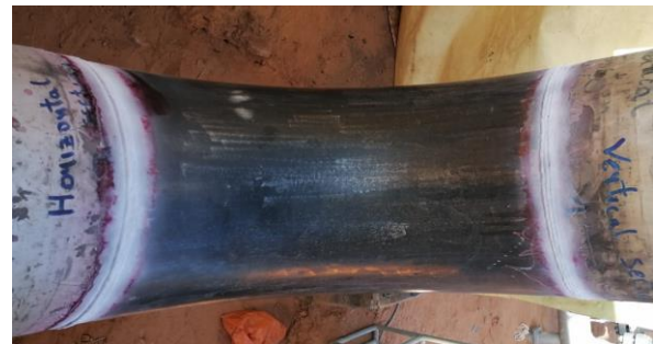
Figure 11. Penetrant test of welded joints: final layers.
