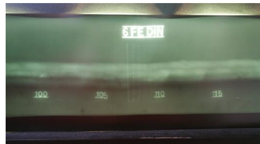
Figure 12. Interpretation of radiographs after welding.
