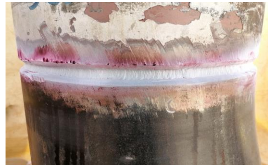
Figure 10. Penetrant tests of welded joints: root pass.
