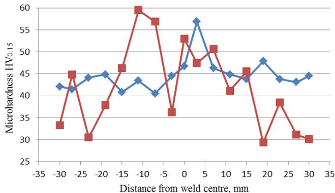
Figure 9. Microhardness distribution at weld face and root side.
