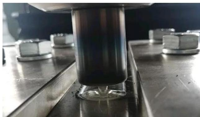
Figure 4. Tool extraction from the welded joint.
