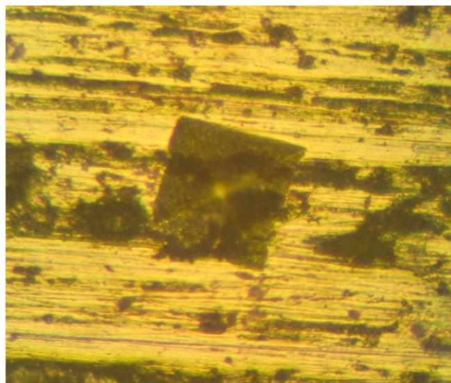
Figure 10. Impression on the sample after measuring the microhardness by Vickers method.
