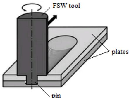
Figure 1. Simplified representation of the FSW lap joint, /12/.
