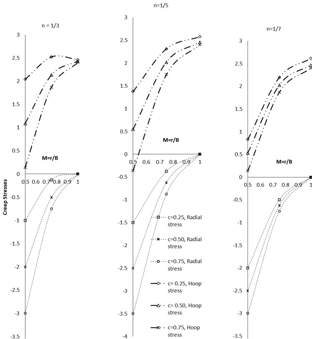
Figure 2. Creep distribution in spherical shell for measure  $n = 1/3, 1/5, 1/7$ .
