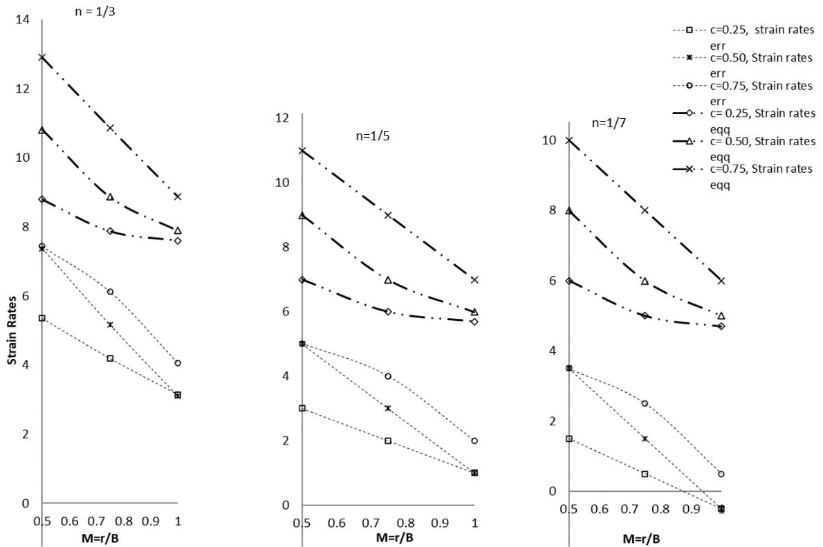
Figure 3. Creep strain rates in spherical shell for measure  $n = 1/3, 1/5, 1/7$ .
