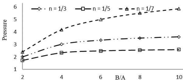
Figure 5. Pressure required for fully plastic state in spherical shell.
