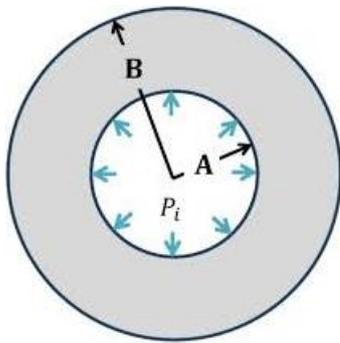
Figure 1. Mathematical model of shell under pressure.
