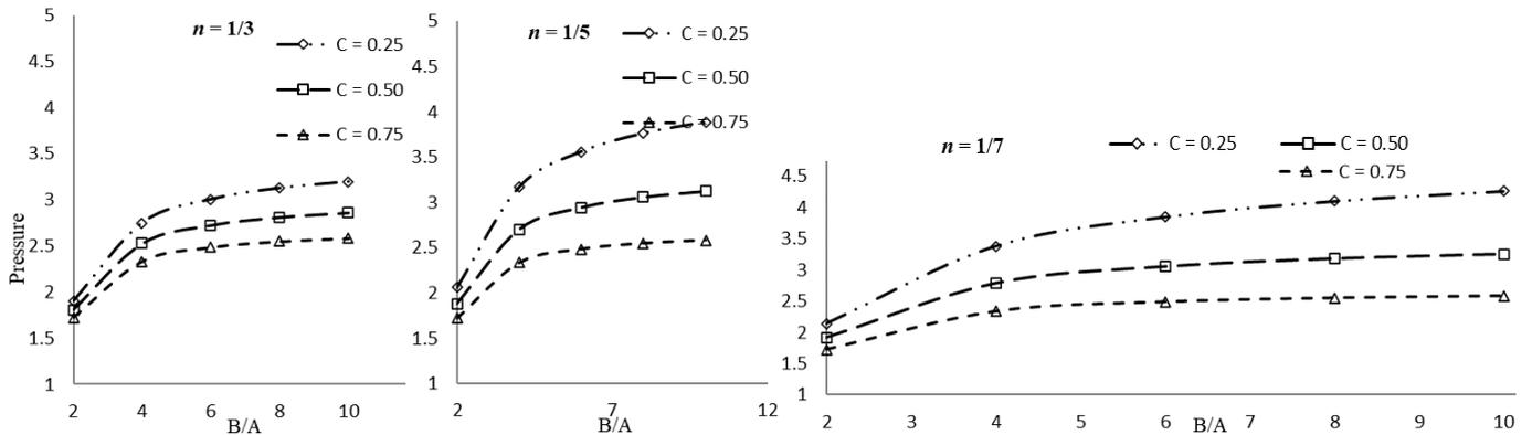
Figure 4. Pressure required for onset of yielding in spherical shell for measure  $n = 1/3, 1/5, 1/7$ .
