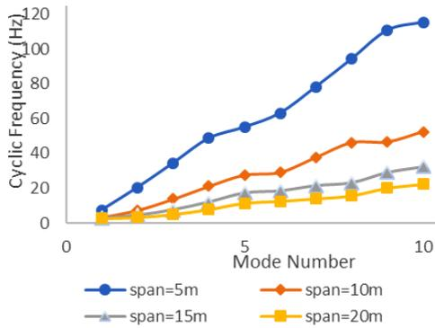
Figure 11. Variation of cyclic frequency with pavement span length.
