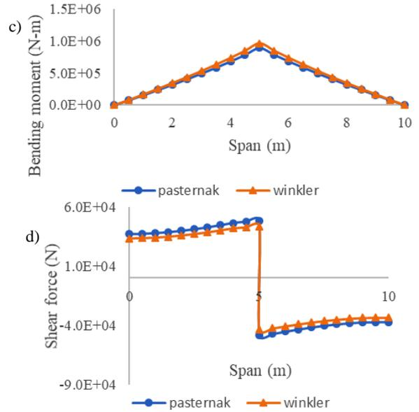
Figure 2a-d. Span length vs. vertical deflection, rotation about z axis, bending moment, and shear force, of rigid pavement resting on Winkler and Pasternak soil foundation.
