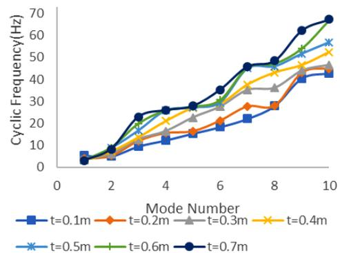
Figure 10. Variation of cyclic frequency with pavement thickness.
