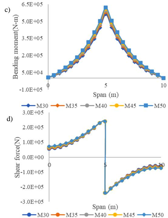
Figure 6a-d. Span length vs. vertical deflection, rotation, bending moment, and shear force with varying modulus of elasticity (E) of pavement.
