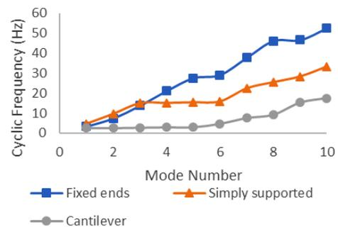
Figure 14. Variation of the cyclic frequency with different boundary conditions.
