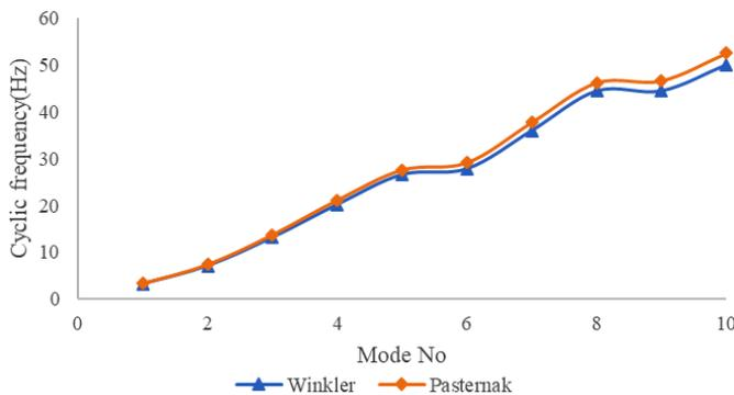
Figure 9. Variation of cyclic frequency for Winkler and Pasternak soil model.
