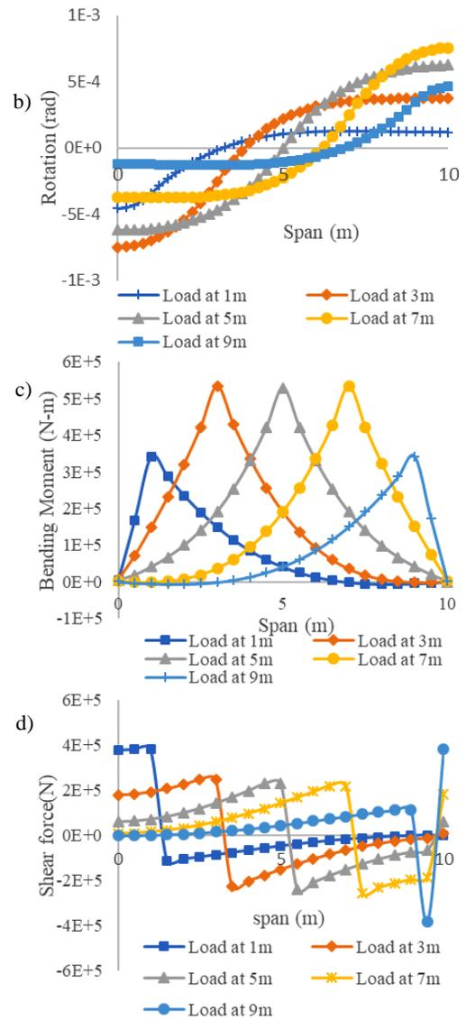
Figure 8a-d. Span length vs. vertical deflection, rotation, bending moment, and shear force with varying load location from the left end along the length.
