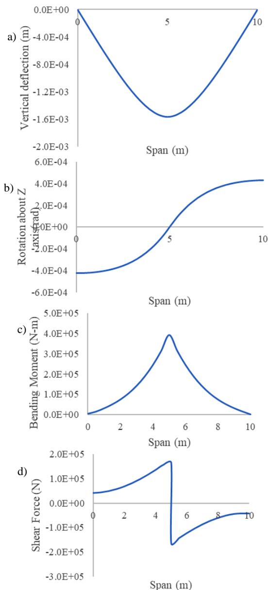
Figure 4a-d. Span length vs. vertical deflection, rotation about z axis, bending moment, and shear force, of rigid pavement resting on two-parameter soil.
