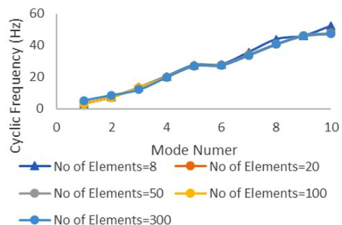
Figure 15. Variation of cyclic frequency with the number of elements.
