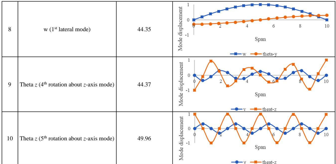
Table 5. Frequency and mode shapes for rigid pavement resting on two-parameter soil model.
