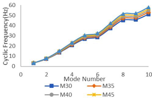
Figure 12. Variation of the cyclic frequency with concrete grade.
