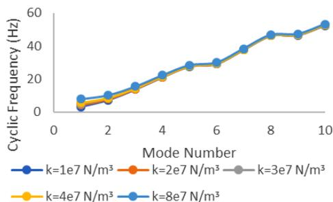
Figure 13. Variation of cyclic frequency with modulus of subgrade,  $k$ .
