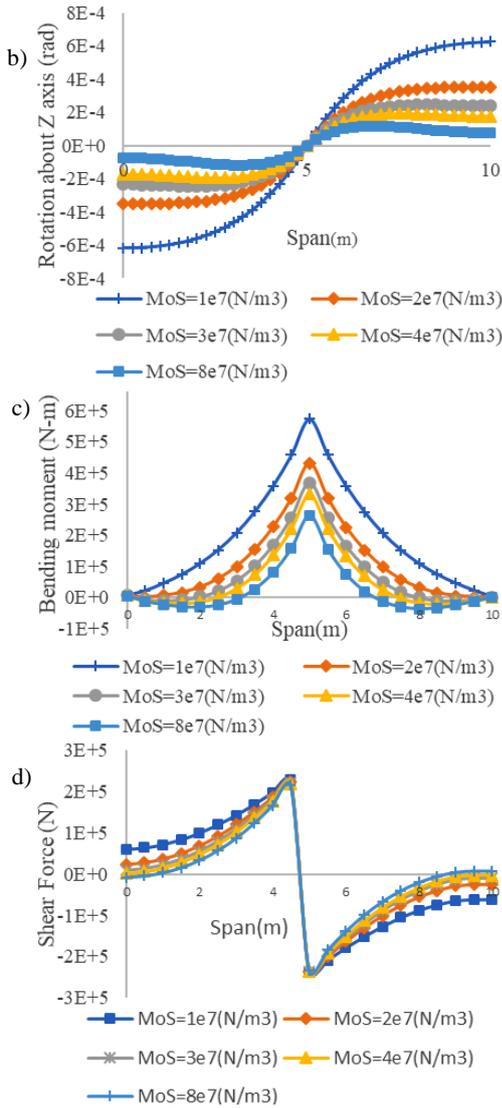
Figure 7a-d. Span length vs. vertical deflection, rotation, bending moment, and shear force with varying modulus of subgrade.
