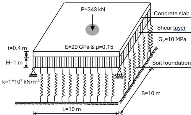
Figure 3. Rigid pavement on two-parameter soil subjected to aircraft loading.
