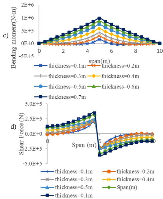
Figure 5a-d. Span length vs. vertical deflection, rotation, bending moment, and shear force with varying thickness.
