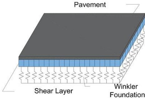
Figure 1. Rigid pavement resting on a two-parameter elastic foundation.
