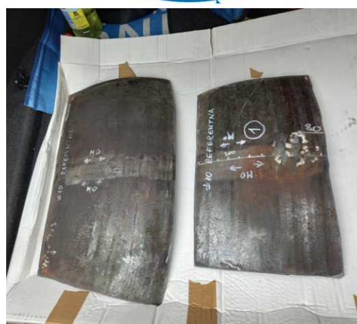
Figure 1. Sampling scheme from the vessel head: tensile specimen -1; Charpy specimen -2; CT specimen -3.
