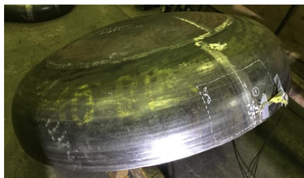
Figure 5. Position of strain gauge on vessel head.
