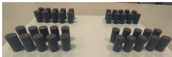
Figure 2. Four sets of compressive specimens.
