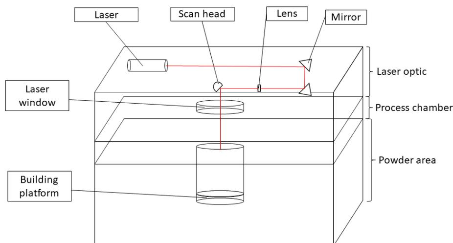
Figure 1. Design of an SLS system. Subdivision of the SLS system into three areas, /11/.
