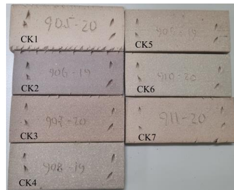
Figure 7. Macro appearance of samples fired at 1250 °C.
