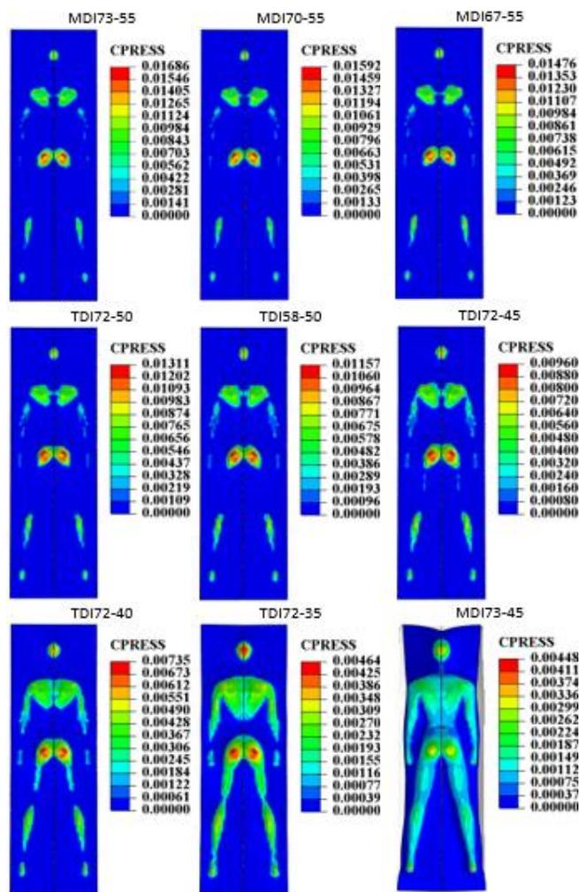
Figure 7. Contact pressure contours (MPa).
