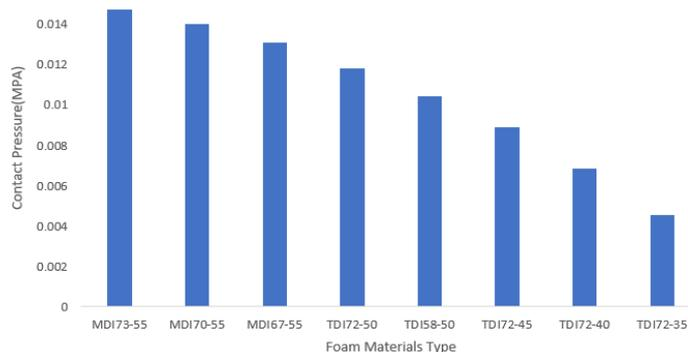
Figure 4. Contact pressure variation in MPa of foam materials (compressive strength).
