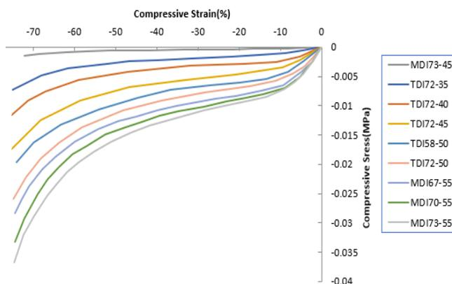
Figure 2. Compressive strength of flexible polyurethane foams.
