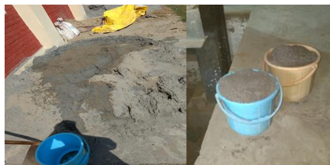
Figure 4. Sample preparation of sand admixed pond ash.
