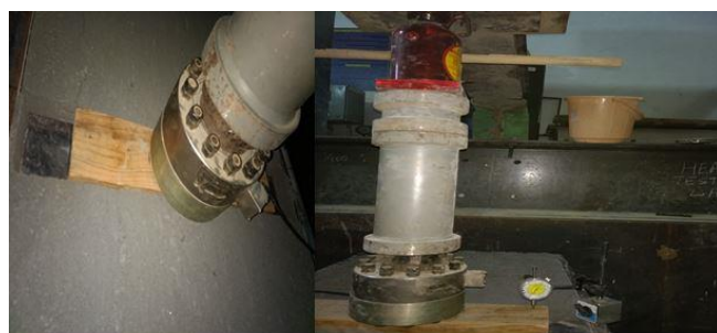
Figure 3. Load application in laboratory plate load test.
