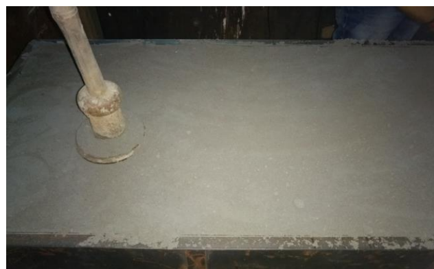
Figure 5. Compaction of sample in test tank.
