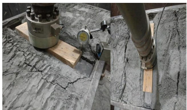
Figure 7. Failure of footing during load application.
