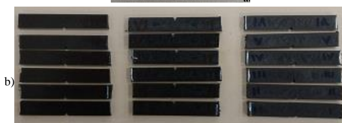
Figure 1. Test specimens prepared for (a) static; and (b) dynamic fracture toughness investigations.
