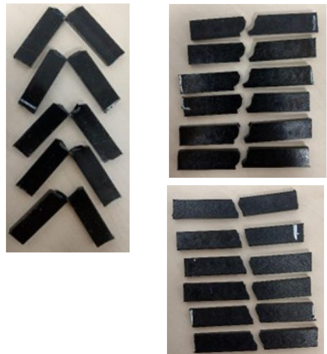
Figure 5. Broken probes from the dynamic fracture toughness test.
