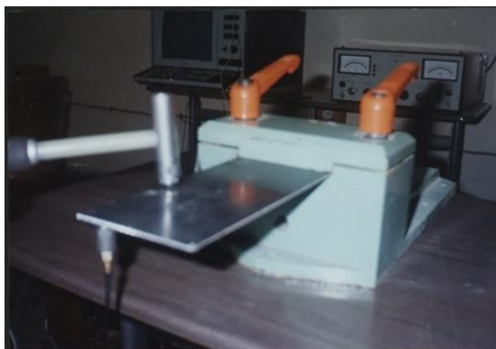
Figure 1. FFT 3550 Bi-channel analyser with impact hammer and accessories (let), and embedding device and tested specimen (right).
