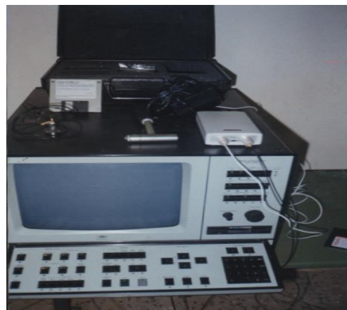
Figure 1. FFT 3550 Bi-channel analyser with impact hammer and accessories (let), and embedding device and tested specimen (right).
