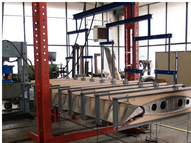
Figure 12. Test assembly with manufactured whiffle-tree.
