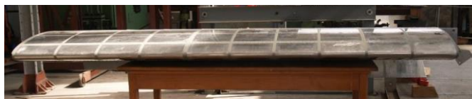
Figure 5. Wing prototype used in the experimental stage.
